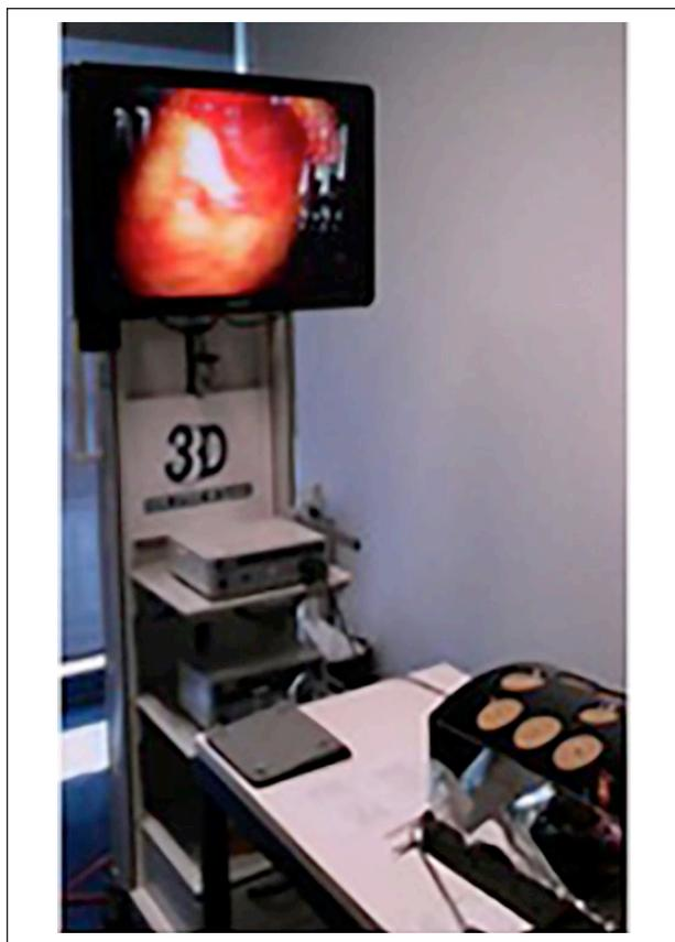
**Figure 2.** Three-dimensional laparoscopic simulator system.
